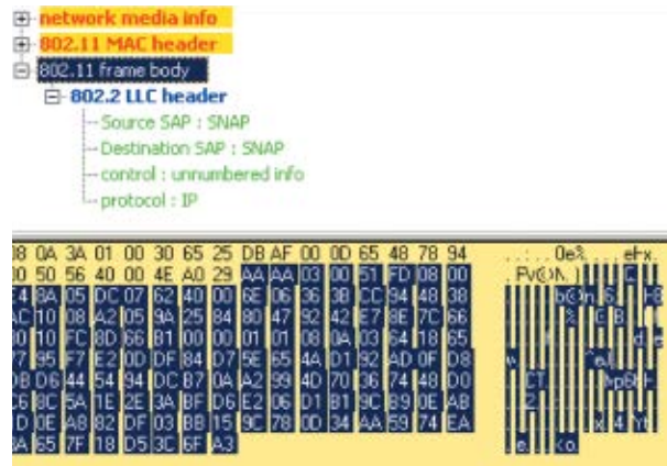
Figure 2. The 802.11 frame body always begins with a SNAP header (for example, AA).
