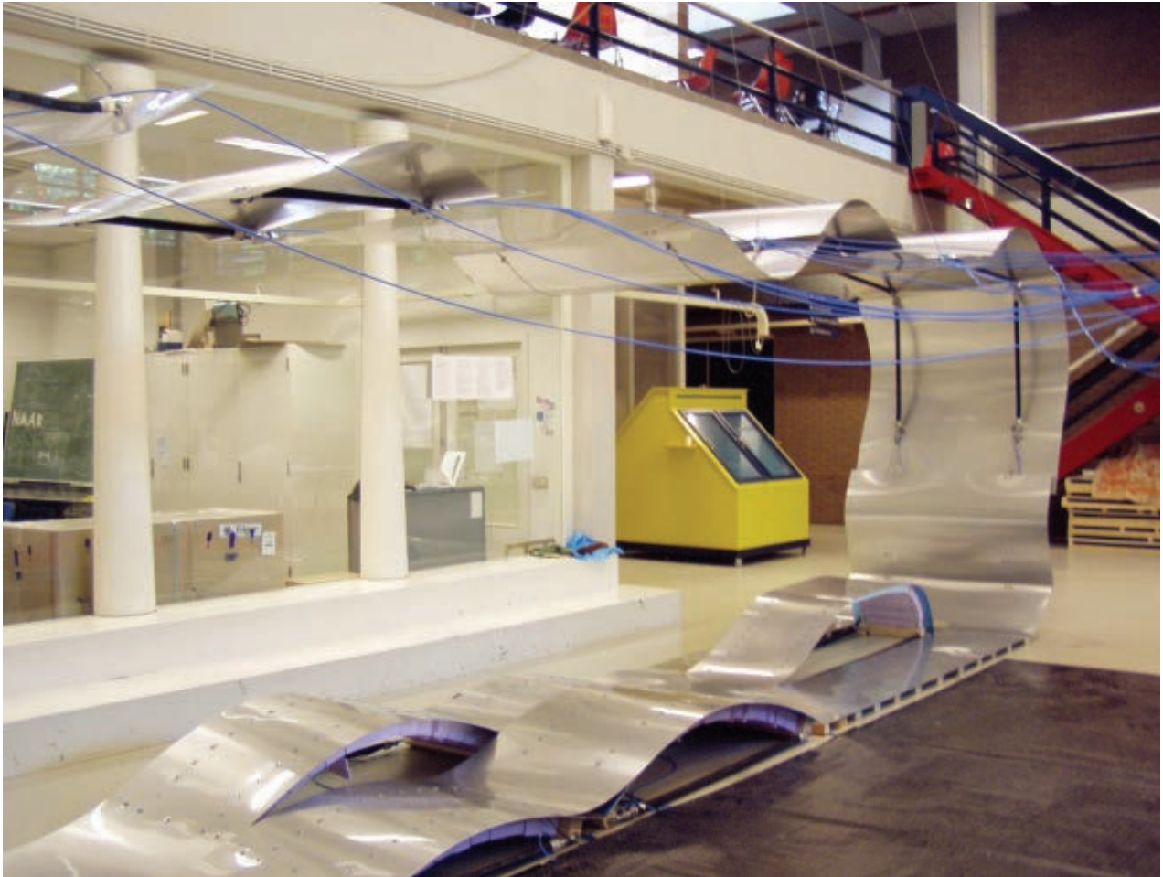
Figure 2. Hylite panels actuated by embedded fluidic Festo Muscles.
