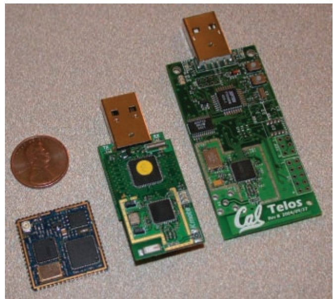
Figure 1: EPIC, KMote, and Telos motes. Each has an 8MHz microcontroller, 10kB of RAM, 48kB of program flash, and a 250kbps radio.
