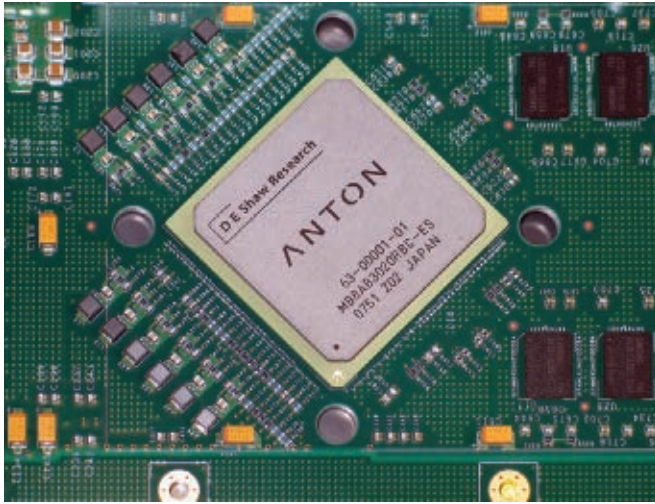
Figure 1: Anton ASIC. One of the first Anton ASICs, which arrived in January 2008.
