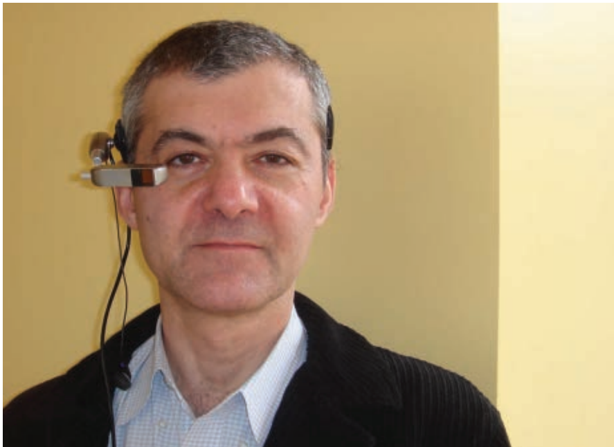
Figure 3: The author Kanevsky, a deaf research scientist, testing IBM's prototype head-mounted display device with IBM's ViaVoice transcription services combined with a human-in-the-loop live transcription service from CaptionFirst, Inc. (www.captionfirst.com/), the first time transcription services were coupled with eyewear and a belt-worn portable computing device.
