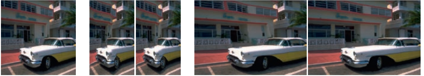
Figure 7: A comparison of results for reduction and expansion of the car image (leftmost) using least cost seam of Equation 5 (left in each pair) and least inserted cost seams of Equation 9 (right in each pair). We discuss image enlarging in Section 4.3.
