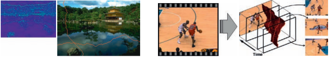
Figure 2: A seam is a connected and monotonic path of low energy pixels (energy shown in small) connecting the two sides of the image either horizontally or vertically (shown in red). On video (right) the sequence of frames is combined to a 3D cube and a 2D monotonic and connected manifold is sought. The intersection of the manifold with each video frame defines the seams on the frame.
