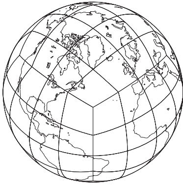
A climate change model of Earth with a quasi-uniform but nonorthogonal quadrilateral grid.
