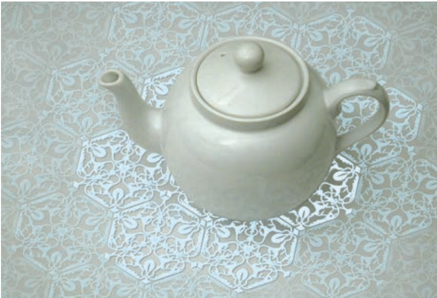
The “History Tablecloth,” developed by the Interaction Research Studio (Goldsmith’s College, University of London), is an example of embedding computing in everyday objects. When items are left on the cloth it begins to glow beneath them, creating a slowly expanding halo. When the items are removed, the glow gradually fades.
