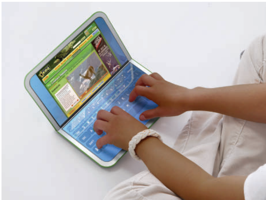
The 2010 version of the One Laptop per Child, the XO-2, will have a foldable e-book form and reduce power consumption to one watt.
