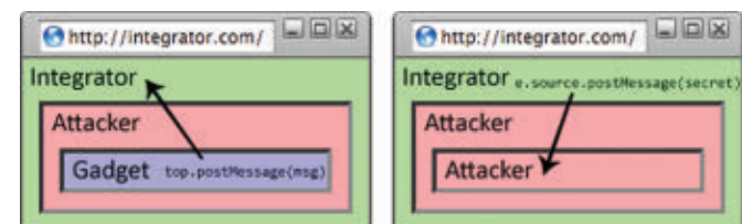
Figure 5: Reply attack. The attacker intercepts the integrator's response to the gadget's message.
