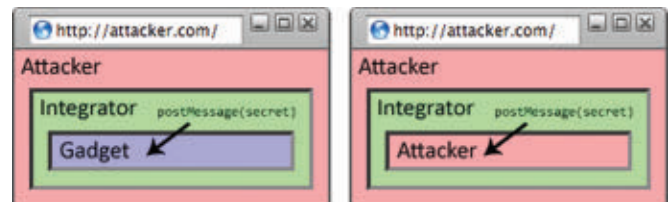
Figure 4: Recursive mashup attack. The attacker navigates the gadget's frame to attacker.com .
