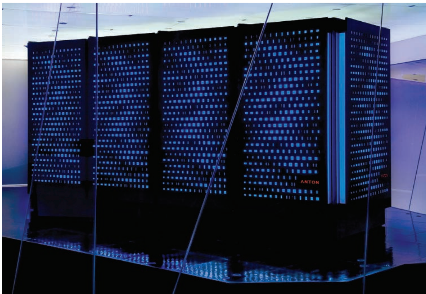
Anton, a massively parallel machine designed to perform molecular dynamic simulations.
