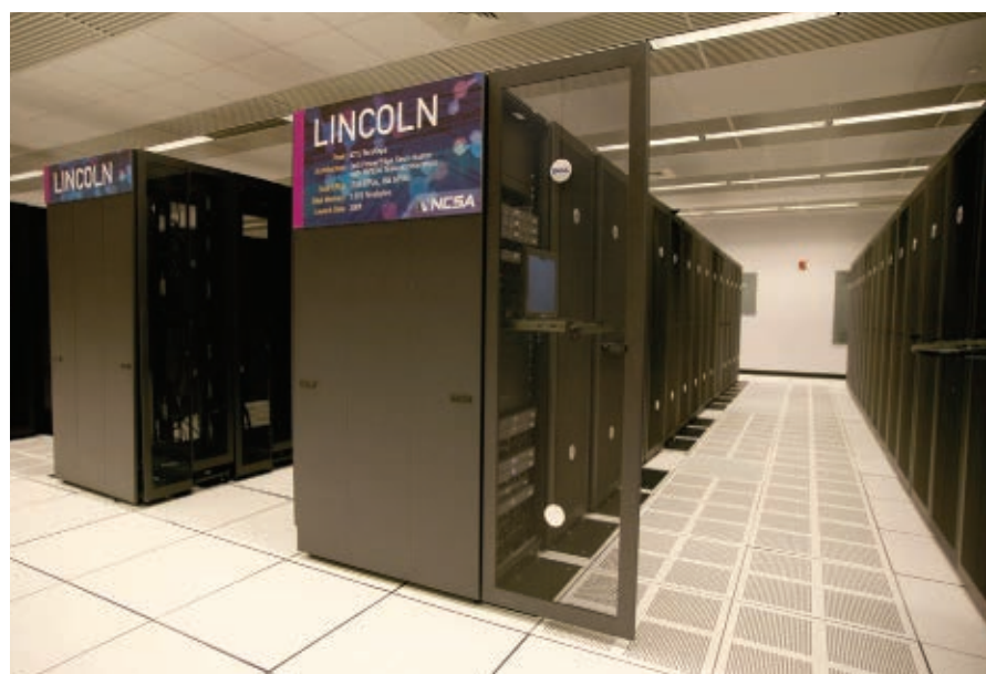
Figure 1. The recently constructed Lincoln GPU cluster at the National Center for Supercomputing Applications contains 1,536 CPU cores, 384 GPUs, 3TB of memory, and achieves an aggregate peak floating-point performance of 47.5TFLOPS.
