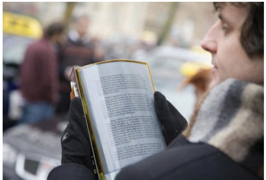
An early prototype of a monochromatic Plastic Logic reading device featuring flexible display technology.
