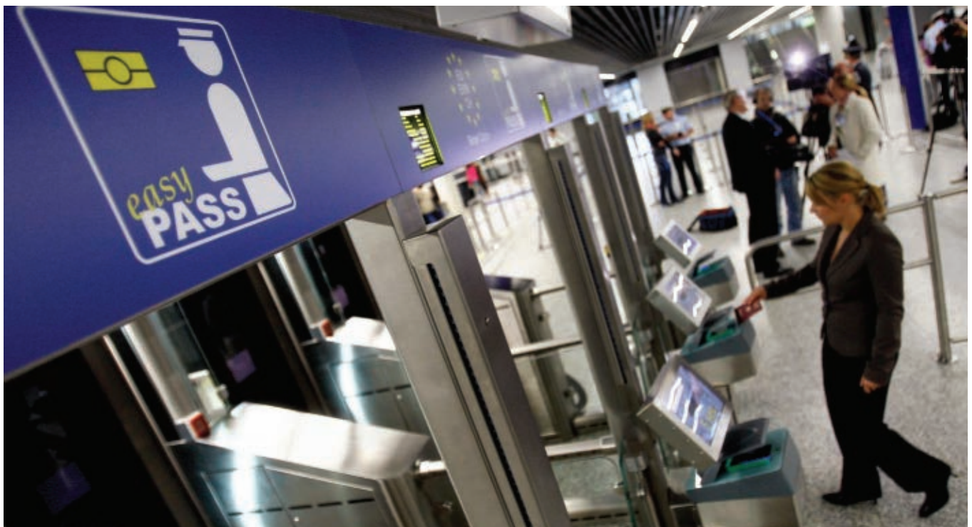
EasyPass, a new automated border control system at Frankfurt International Airport, scans passenger biometric data and compares it to data from the person's e-passport.
