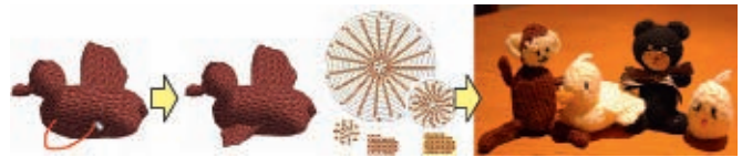
Figure 22. Knitty system allows the user to design an original knitted toy by simply drawing the desired silhouette.
