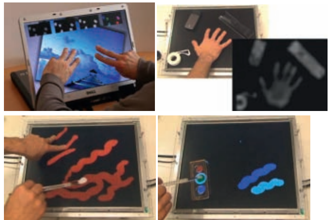
Figure 1. ThinSight brings the novel capabilities of surface computing to thin displays. Top left: photo manipulation using multiple fingers on a laptop prototype (note the screen has been reversed in the style of a Tablet PC). Top right: a hand, mobile phone, remote control and reel of tape placed on a tabletop ThinSight prototype, with corresponding sensor data far right. Note how all the objects are imaged through the display, potentially allowing not only multitouch but tangible input. Bottom left and right: an example of how such sensing can be used to support digital painting using multiple fingertips, a real brush and a tangible palette to change paint colors.
