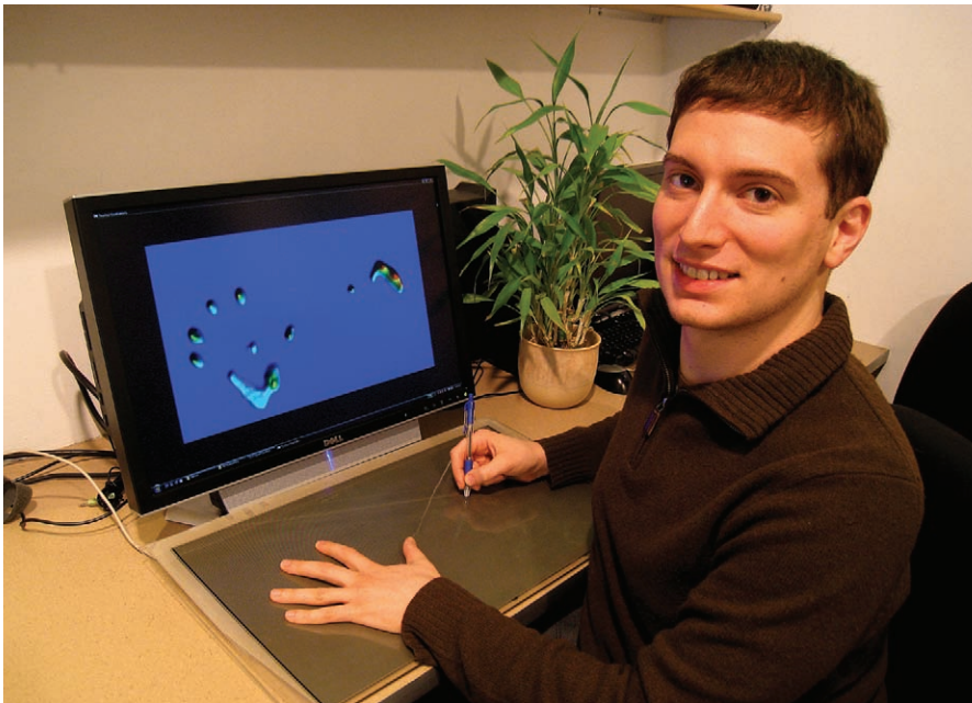
Interpolating force sensitive resistance (IFSR), a multitouch input technology developed at New York University’s Media Research Lab. In this demo, Ilya Rosenberg demonstrates a 24-inch Touchco IFSR sensor that serves as an interactive desktop surface.
