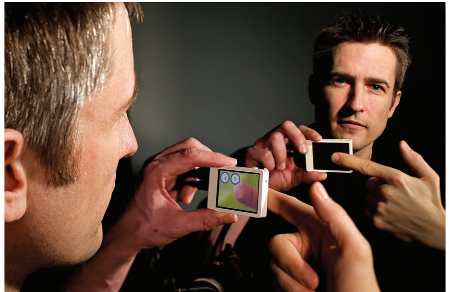
NanoTouch, a back-of-device input technology for very small screens on mobile devices and electronic jewelry. The technology demonstrated here by Patrick Baudisch was developed at Microsoft Research and Hasso Plattner Institute.
