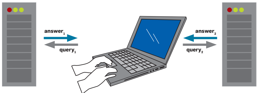
Two-server information-theoretic PIR scheme. To retrieve a database record, the user queries two servers, each of which stores a copy of the database, but individual queries carry no information about what the user is after. The desired record is obtained from the servers’ combined responses.
