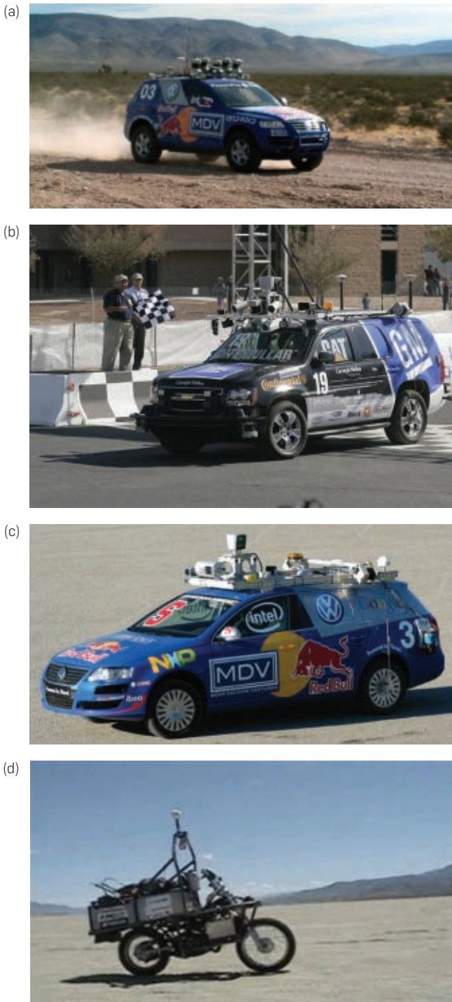
Figure 1. Autonomous robots in the DARPA Challenges: (a) Stanford's robot Stanley, winner of the Grand Challenge; (b) CMU's Boss, winner of the Urban Challenge (photograph courtesy of Carnegie Mellon University, Tartan Team); (c) Junior, runner-up in the Urban Challenge; and (d) UC Berkeley's Ghost rider motorcycle (photograph courtesy of Anthony Levandowski, Blue Team).
