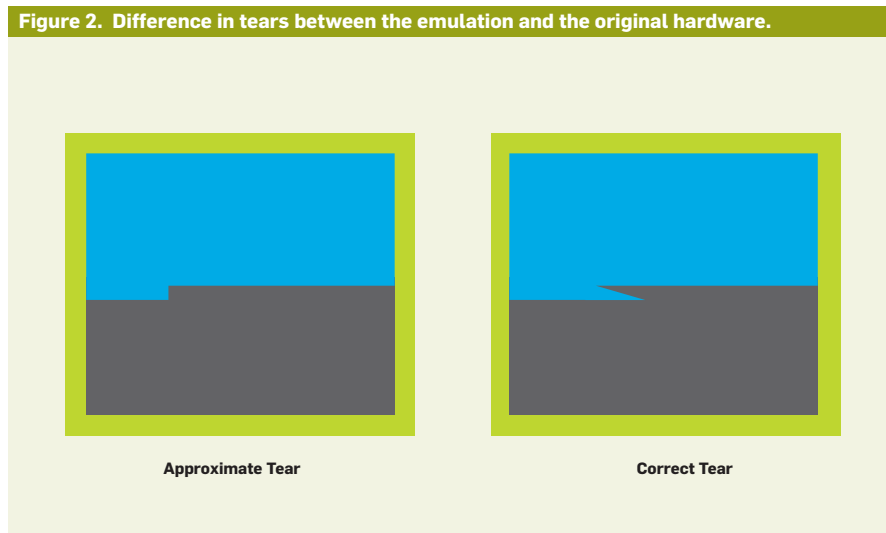
Figure 2. Difference in tears between the emulation and the original hardware.
