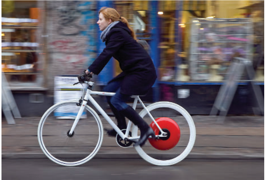
With the Copenhagen Wheel, an ordinary bicycle is transformed into a hybrid electronic vehicle that records road conditions, traffic congestion, and pollution levels in real time.
