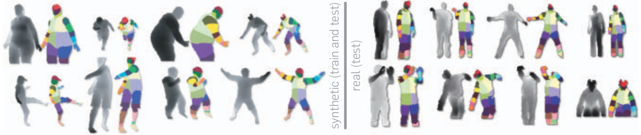
Figure 4. Synthetic and real data. Pairs of depth image and ground truth body parts. Note wide variety in pose, shape, clothing, and crop.
