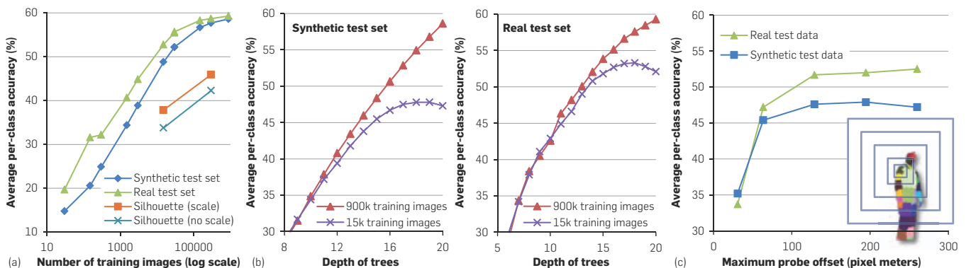
Figure 8. Training parameters versus classification accuracy. (a) Number of training images. (b) Depth of trees. (c) Maximum probe offset.
