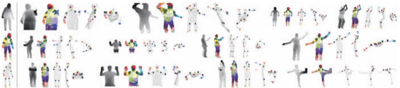
Figure 7. Example inferences. Synthetic (top row), real (middle), and failure modes (bottom). Left column: ground truth for a neutral pose as a reference. In each example, we see the depth image, the inferred most likely body part labels, and the joint proposals shown as front, right, and top views (overlaid on a depth point cloud). Only the most confident proposal for each joint above a fixed, shared threshold is shown.
