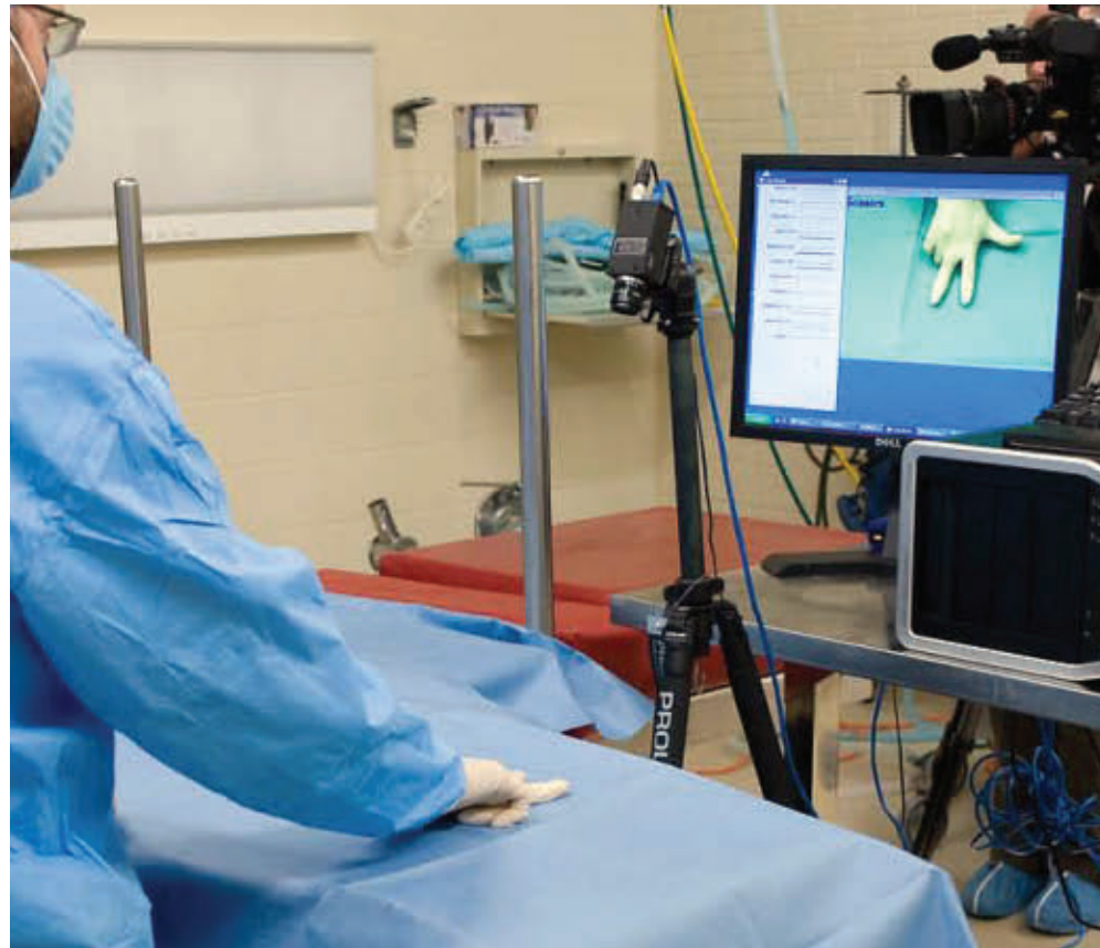
The surgeon requests scissors from Gestonurse using a hand signal recognized by the camera above the surgical bed.
