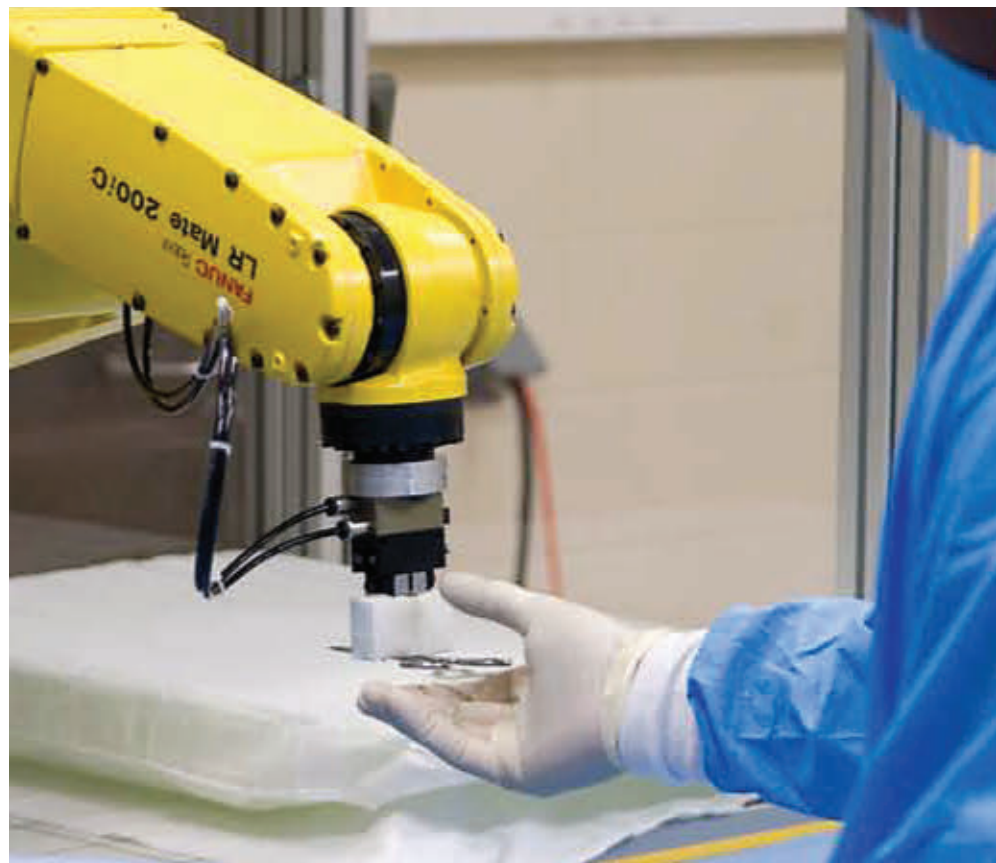
Gestonurse safely hands off a surgical scissors to the surgeon requesting it.
