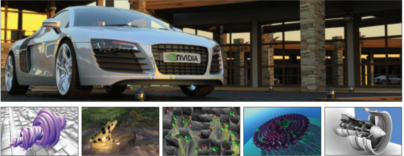
Figure 1. Images from various applications built with OptiX. Top: Physically based light transport through path tracing. Bottom: Ray tracing of a procedural Julia set, photon mapping, large-scale line of sight and collision detection, Whitted-style ray tracing of dynamic geometry, and ray traced ambient occlusion. All applications are interactive.
