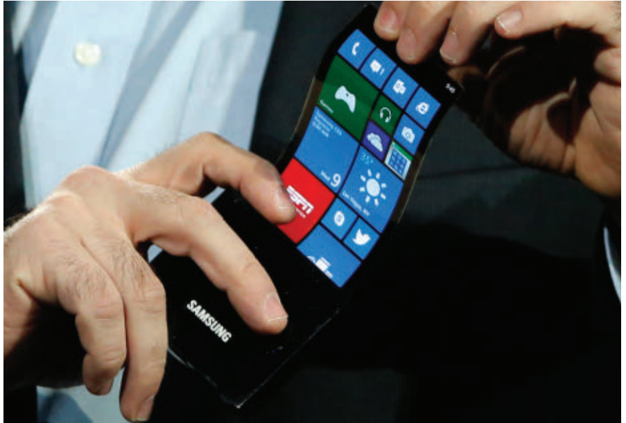
A prototype of Samsung's flexible smartphone, shown at the International Consumer Electronics Show in January 2013.
