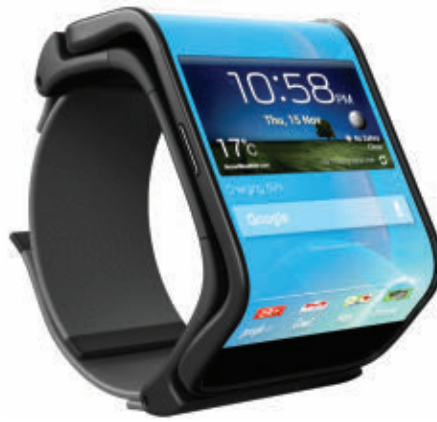
The Limbo flexible concept smartphone, made to be used as a standard handset or bent around the arm and worn in wristwatch fashion.
