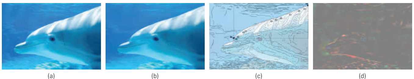
Figure 7. Automatic vectorization of a bitmap image: (a) original bitmap, (b) automatic vectorization, (c) diffusion curves, and (d) RGB difference (amplified by 4). Note that the most visible error occurs along edges (d), most probably because, through vectorization, we change their location.
