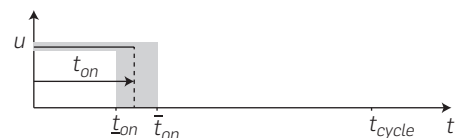
Figure 5. Range of times [t_{on}, \bar{t}_{on}] when the charge pump is switched off. The mode both_active is not considered in this figure.
