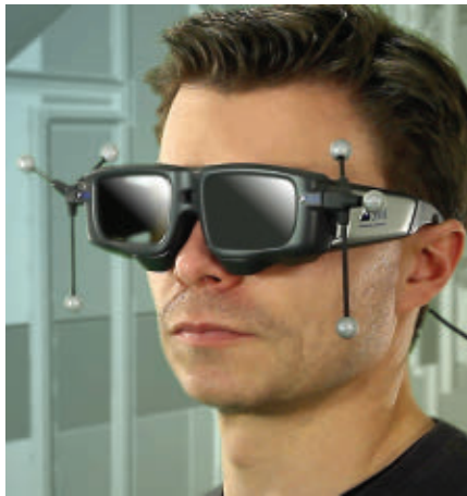
Unlike gaze tracking systems that do not require additional peripherals, SensoMotoric Instruments GmbH's 3D Eye Tracking system has users wear specialized eye tracking glasses.
