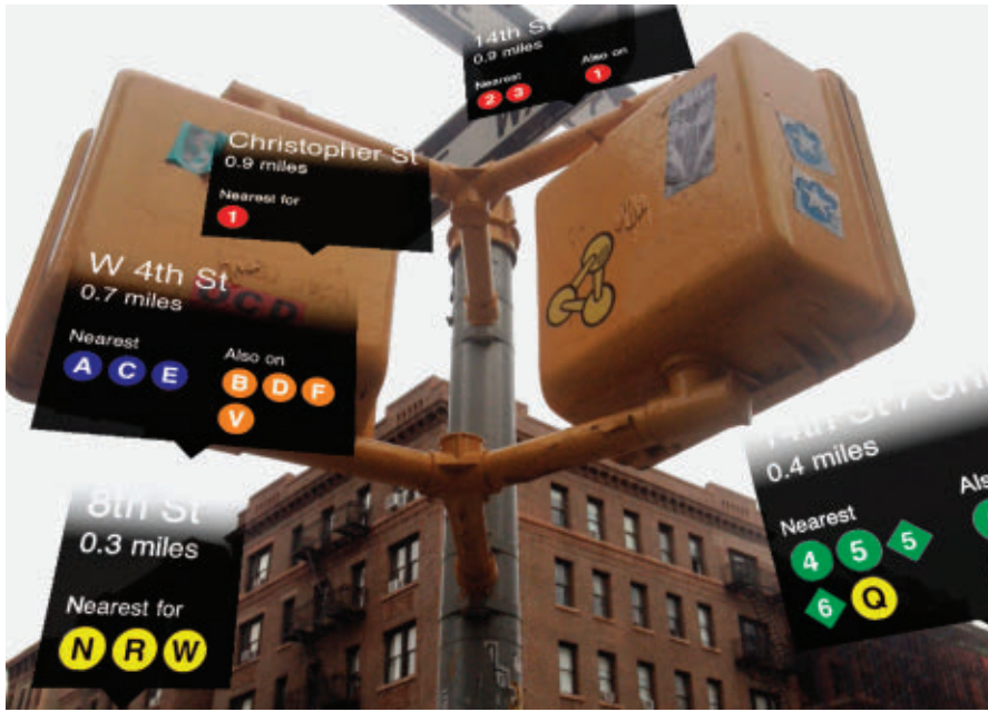
An AR browser view of a New York City street intersection with subway information and distance overlays displayed.
