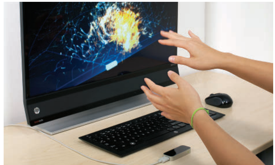
The Leap Motion controller tracks users' hand movements.
