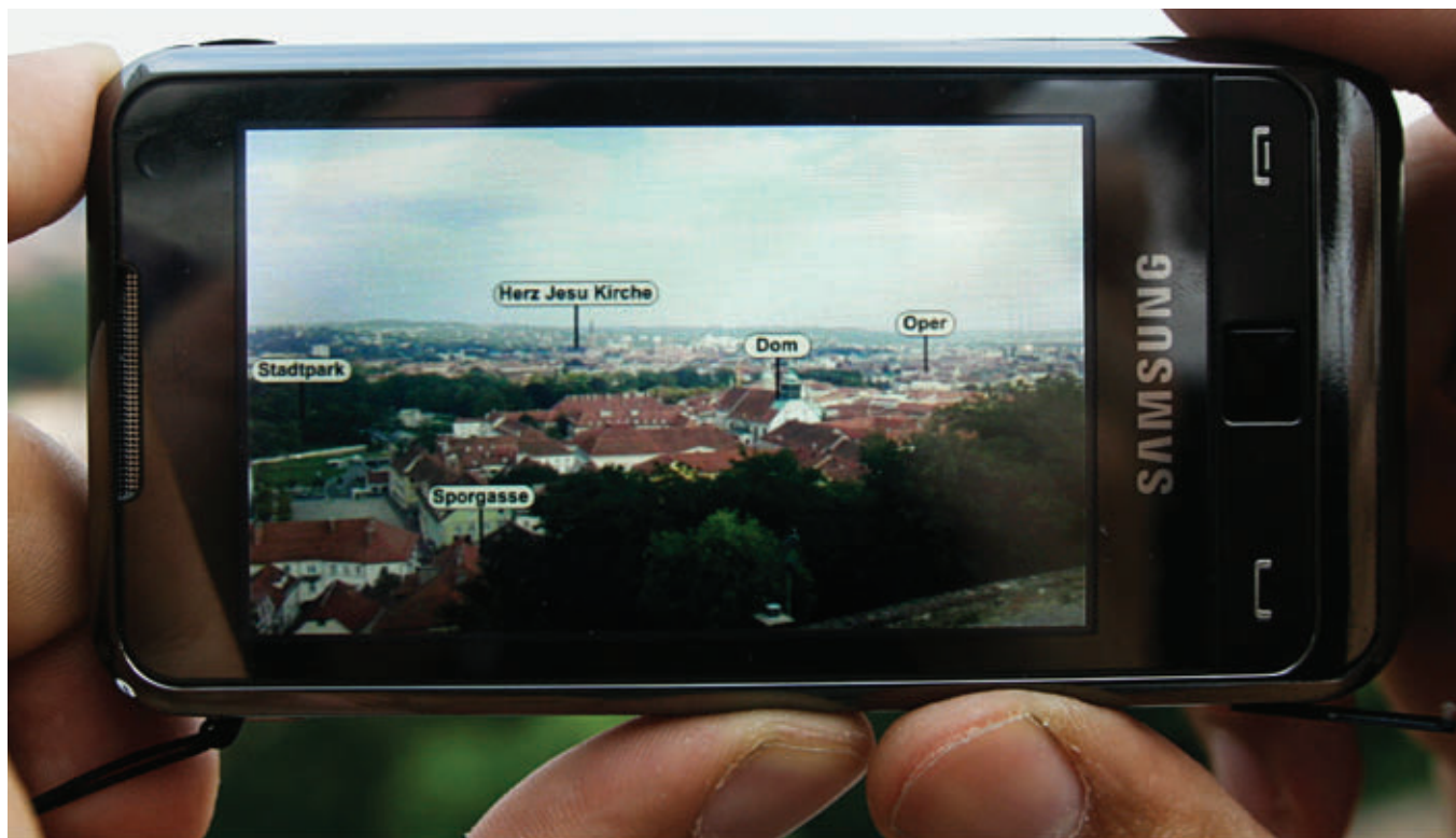
An AR browser application links geographical location of the real world (point of interest) with digital content (text labels): the information is spatially registered in the environment when seen through the camera view of a smartphone.
