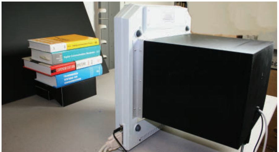
At top, a diagram of how Bell Labs’ lensless camera works: its single-pixel sensor is arrayed behind an aperture assembly that can create a matrix of apertures of varying opacity, so multiple measurements of light data can be conducted at once. Bottom, the lensless camera (black box) undergoes testing.
