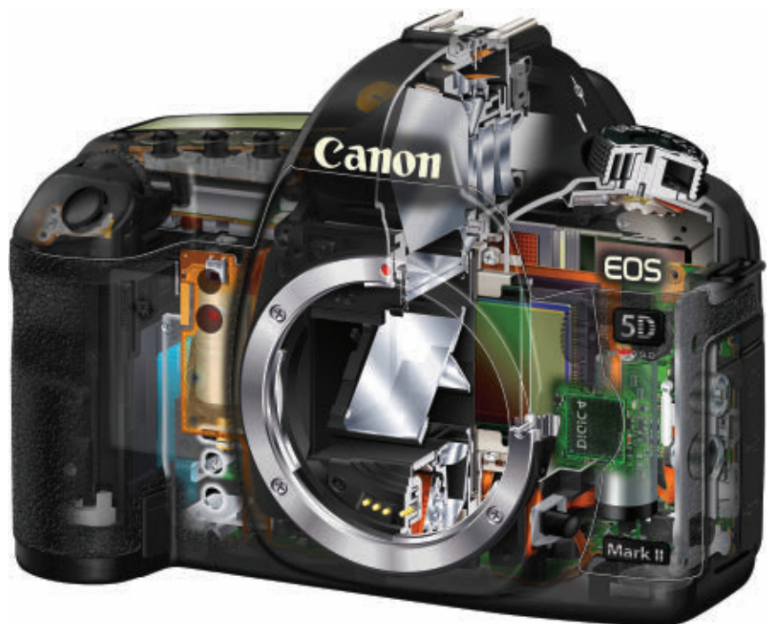
A cutaway view of the Canon EOS 5D Mark II camera body.
