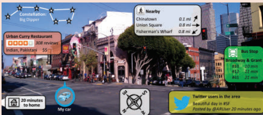
Figure 3. Multi-application AR. Emerging and future AR platforms will support multiple applications running simultaneously, sharing input and output devices, and exposing data and APIs to each other. In a multi-application AR system, applications like those depicted in this mockup will share output devices, including displays, audio output, and haptic feedback. Conflicts among these applications can result in security concerns.
