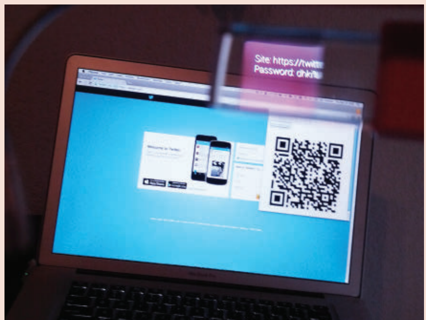
Figure 5. Prototype AR Password Manager. Our Chrome extension (background) displays a QR code representing the current website. In response to the voice command “find password,” our Google Glass application (foreground) scans this QR code and displays the stored password for that site privately in the heads-up display.
