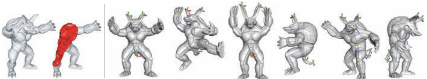
Figure 7. The human skeleton embedded in the Armadillo does not control the tail or the ears, but points are easily added for additional expressiveness in each pose. Left: a cutaway of the Armadillo shows the graded tet mesh produced by TetGen. The inner tetrahedra are much larger than those near the surface. This keeps the discretization complexity reasonable.
