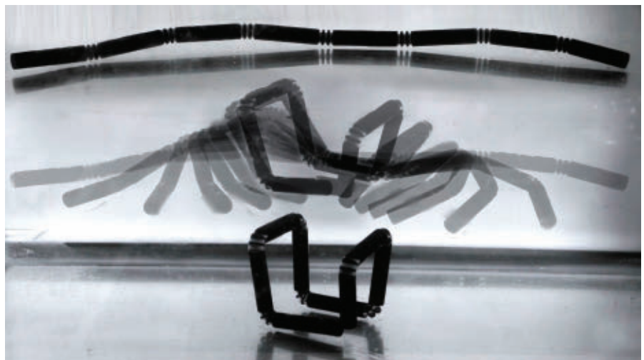
Above, a basic depiction of how a 3D printed object that changes shape or self-assembles over time becomes a 4D printed object. Below, one of Skylar Tibbits’ 4D objects; this 3D printed “self-folding straw” starts out as a cable-like structure, but it assembles itself into a pre-programmed shape when it encounters water.
