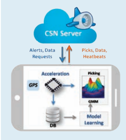
Figure 4. The CrowdShake app processes sensor data locally on an Android phone or tablet, sends pick messages during potential quakes, receives alerts, and responds to data requests.
