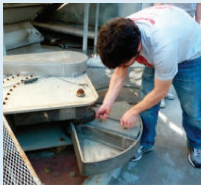
Figure 6. Eccentric weights oscillate Millikan Library, showing CSN hardware is sensitive to resonant frequencies in buildings.
