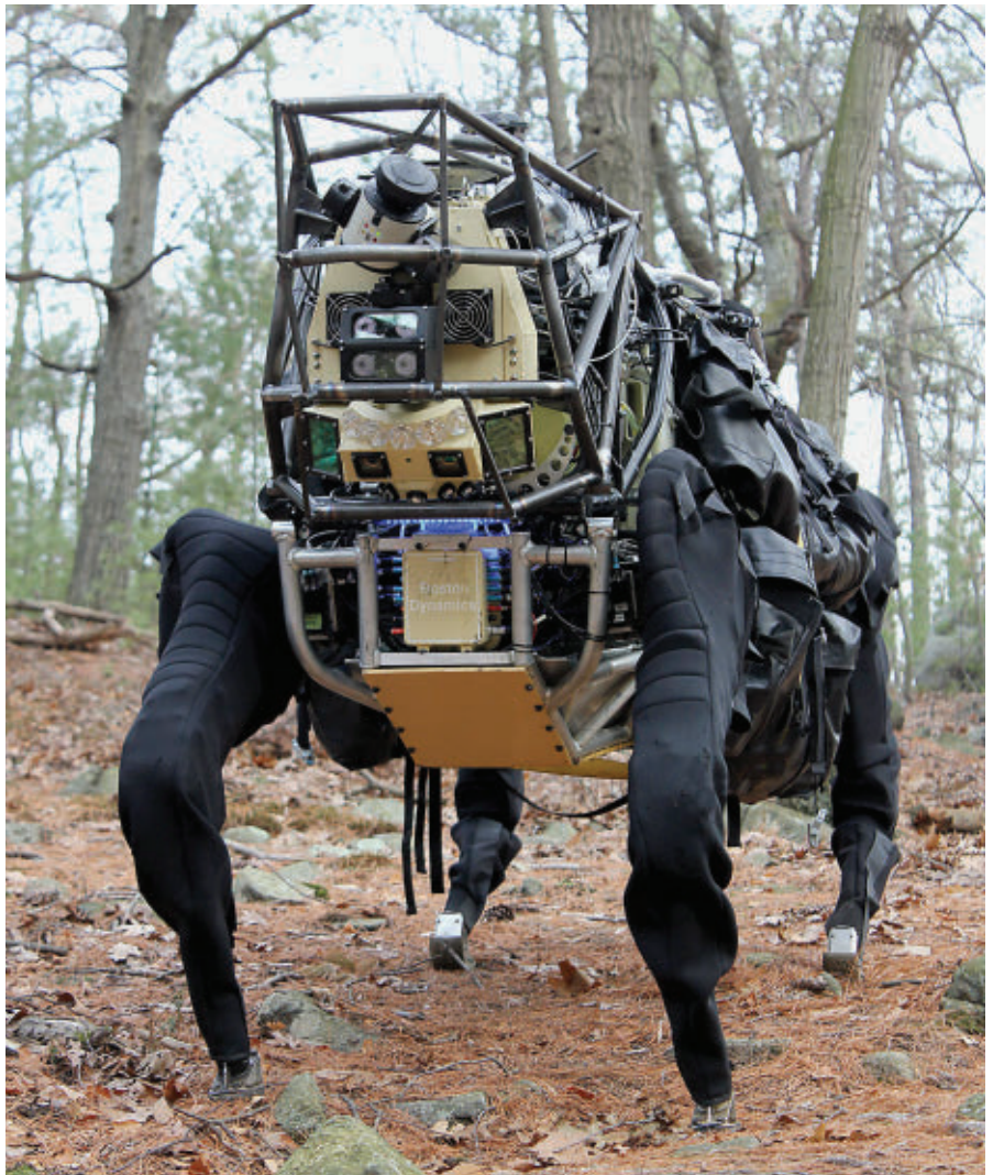
DARPA's semi-autonomous Legged Squad Support System (AlphaDog) was developed from a decade of research on perception, autonomy, and mobility.
