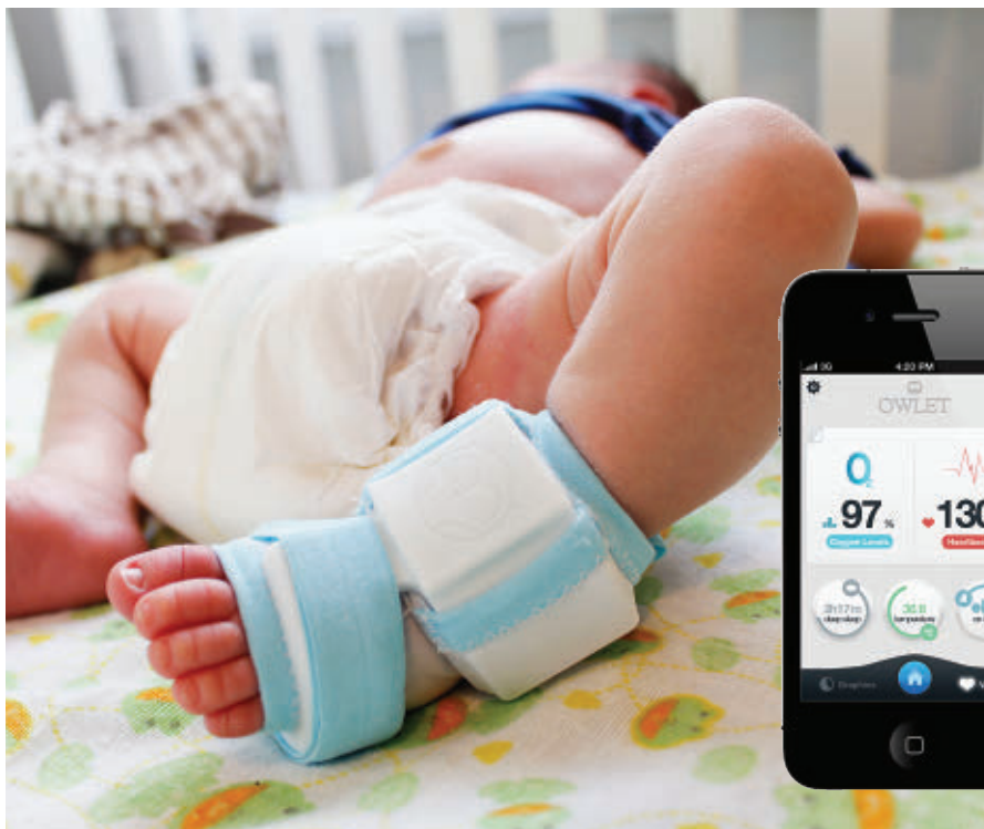
The Owlet Smart Sock wirelessly transmits a child’s health data to a parent’s smartphone via Bluetooth 4.0.
