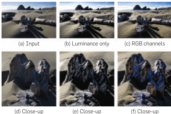
Figure 8. Filtering only the luminance (b) preserves the original colors in (a), while filtering the RGB channels (c) also modifies the color contrast ( \alpha = 0.25, \beta = 1, \sigma = 0.4 ).
