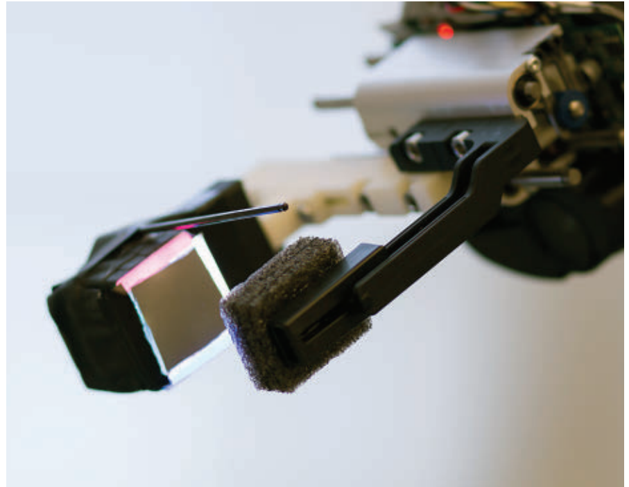
Equipped with the high-resolution GelSight tactile sensor, a robot can grasp a cable and plug it into a USB port.
