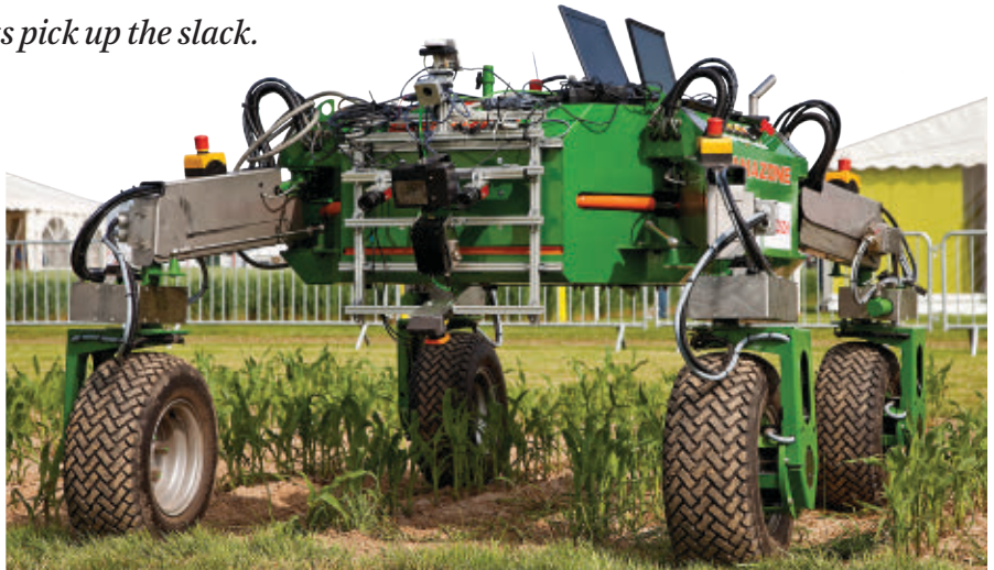
The BoniRob is a multipurpose robotic platform for agricultural applications featuring independently steerable drive wheels and adjustable track width.
