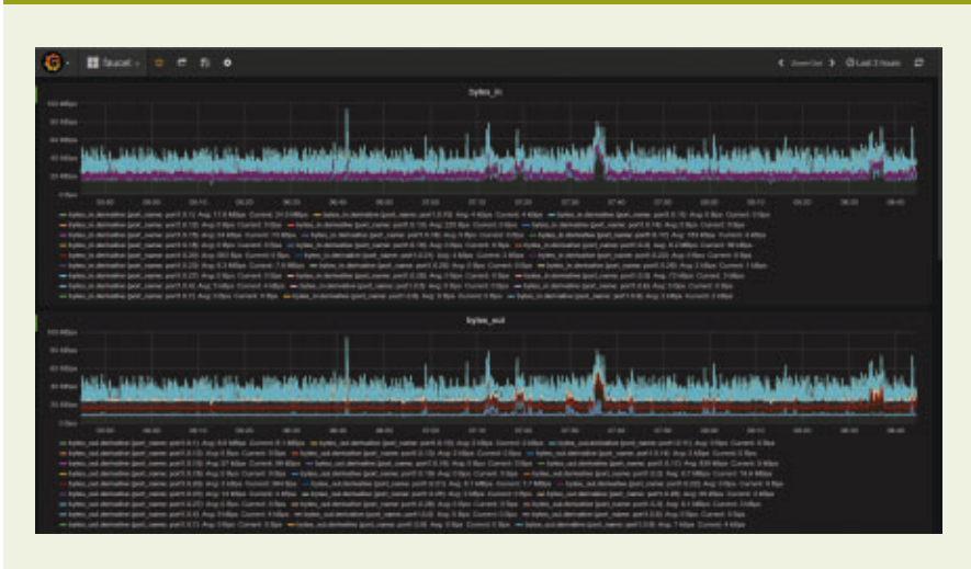
Figure 3. Using Faucet and Grafana to construct dashboards and run queries.
