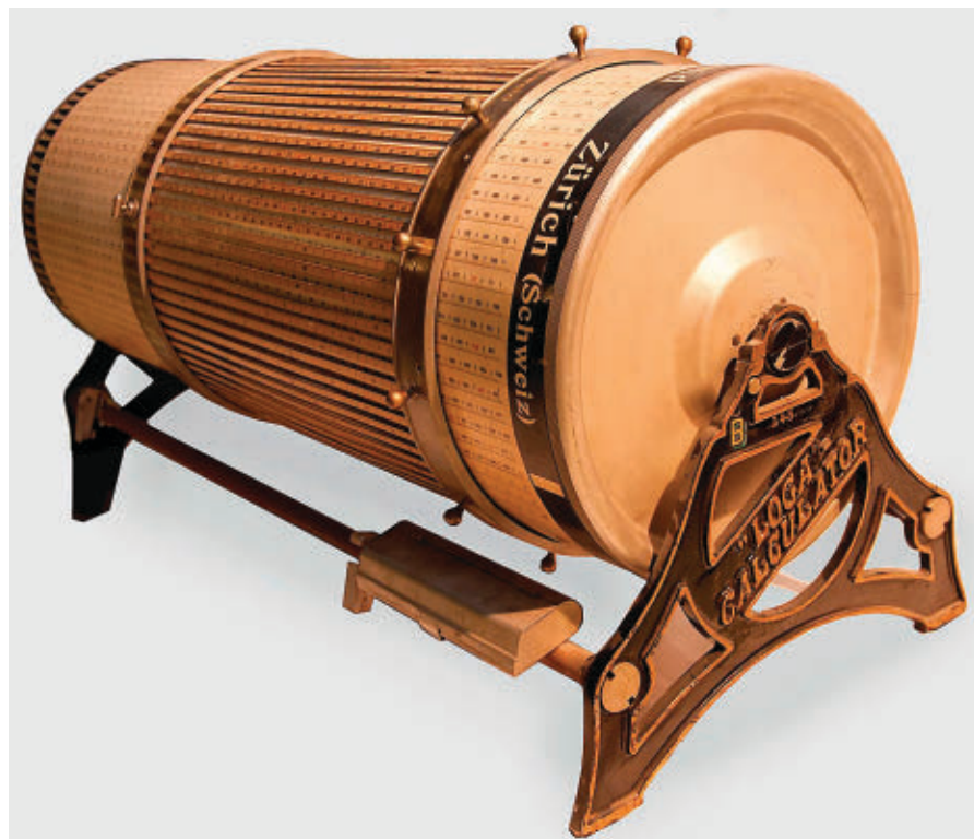
Figure 9. The world’s largest mass-produced cylindrical slide rule from Loga Calculator (circa 1912), Zürich/Uster, Switzerland; length of scale: 24 meters. Multiplication is reduced to addition and division to subtraction in the same way traditional slide rules work. These devices were common in banks and insurance companies worldwide. Courtesy of UBS, Basel, Switzerland.
