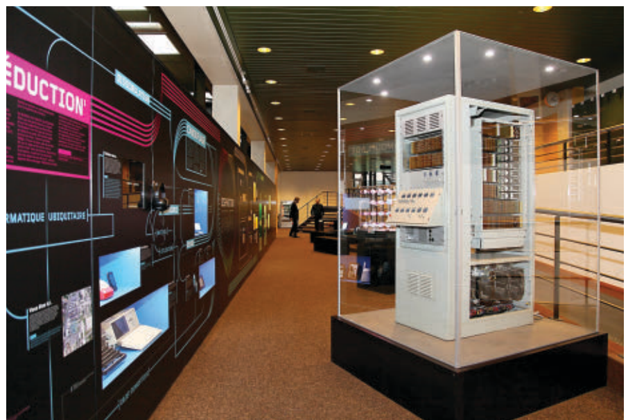
Figure 17. Swiss transistorized computer Cora developed and manufactured by Contraves AG, Zürich, in 1963 originally for military purposes as a fire-control calculator. Courtesy of Musée Bolo, Ecole polytechnique fédérale Lausanne, Switzerland.
