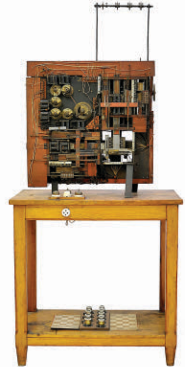
Figure 10. Early electromechanical chess automaton (1912) by Torres Quevedo; unlike Wolfgang von Kempelen’s machine, it is an authentic automaton without hidden human chess player. Courtesy of Museo Leonardo Torres Quevedo, Universidad Politécnica de Madrid, Spain.
