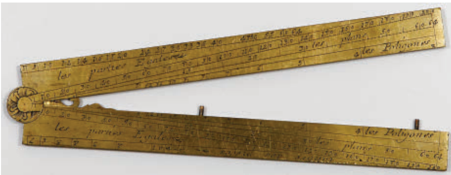
Figure 2. Sector, a universal calculating instrument developed in the 16 th century containing various scales (such as trigonometric) depending on scope; a pair of dividers is necessary for multiplication or division. The sectors are based on the Thales' intercept theorem on intersecting lines. 1,25 Courtesy of the Collection of Astronomical Instruments, ETH Library Zürich, Switzerland.
