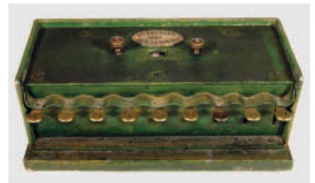
Figure 4. Early key-driven adding machine, or so-called "direct adding machine," developed by Jean-Baptiste Schwilgué of Strasbourg, patented in 1844; pressing a key causes the corresponding number to be stored in the register, making addition very quick. Courtesy of the Collection of Astronomical Instruments, ETH Library Zürich, Switzerland.
