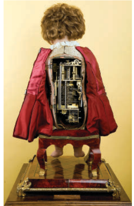
Figure 3. Early programmable handwriting automaton with internal mechanics built by Pierre Jaquet-Droz, 18 th century; the text (up to 37 characters) is stored on cam plates. Courtesy of Musée d'Art et d'Histoire, Neuchâtel, Switzerland.
