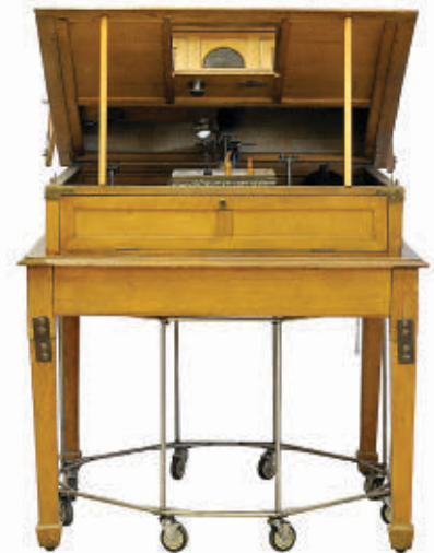
Figure 11. Second automatic chess endgame machine by Torres Quevedo, playing with king and rook (automaton) vs. king (human player). Courtesy of Museo Leonardo Torres Quevedo, Universidad Politécnica de Madrid, Spain.
