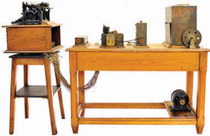
Figure 12. Torres Quevedo's electromechanical arithmometer (1920), typewriter controlled, with conditional branching, based on Charles Babbage's analytical engine. Courtesy of Museo Leonardo Torres Quevedo, Universidad Politécnica de Madrid, Spain.
