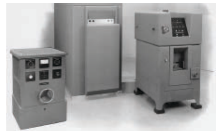
Figure 16. Zuse’s program-controlled parallel decimal electromechanical “calculating punch” M9 manufactured for Remington Rand, Zürich; combined with punched-card machines, the M9 was used for multiple applications (such as for accountancy and statistics). Courtesy of Max Forrer, Oberhelfenschwil, Switzerland.
