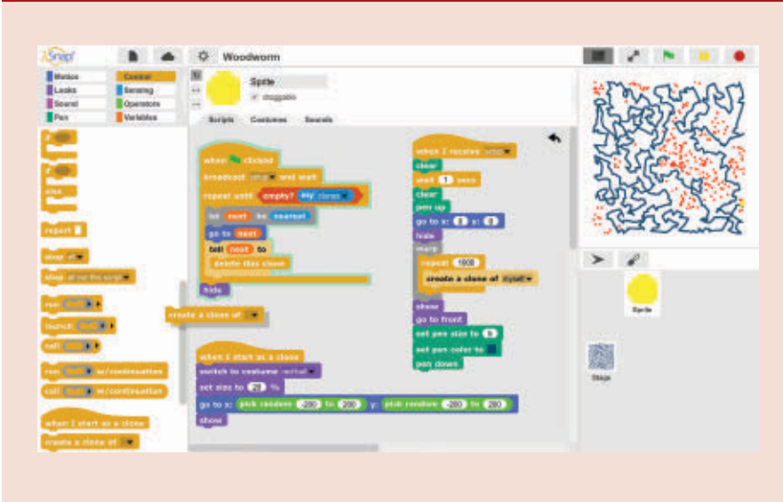
Figure 1. Snap! is an example of a blocks-based programming environment. Users drag blocks from a palette of programming elements (left) into workspace (center), where blocks can be assembled into programs. Snap! also provides an output window (top-right) and a sprite picker (bottom-right).
