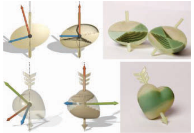
Figure 4. Asymmetric “Ellipsoid” and “Heart”: (Left) Unstable input designs with misaligned principal axes. (Middle) Optimized results after hollowing: for the “Ellipsoid”, a cross-section is shown. The dominant principal axis (red) aligns with the spin axis. Opaque surfaces indicate the boundary of the void space. (Right) Fabricated results with hollowing.
