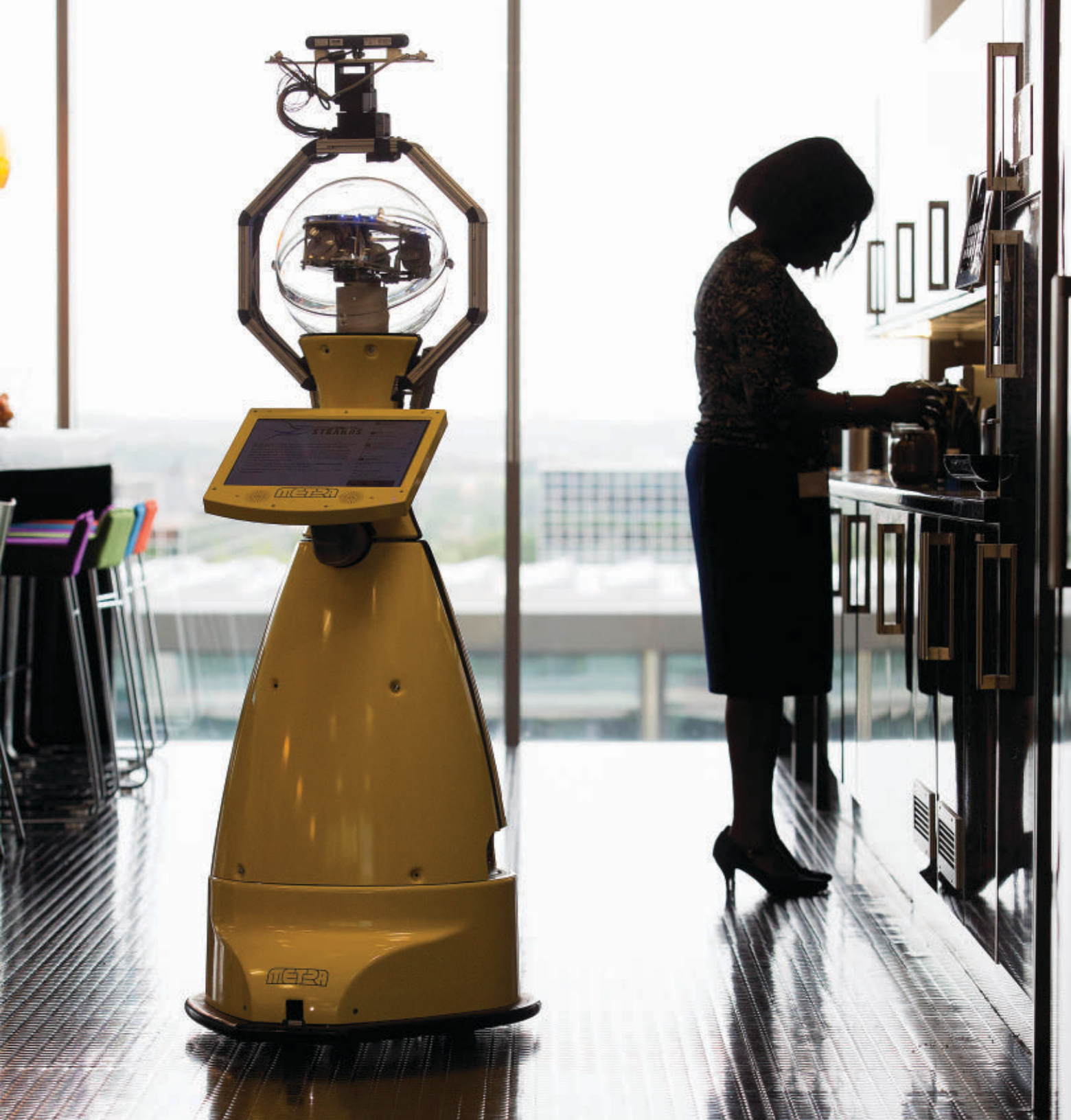
Autonomous robot (Betty) developed at the University of Birmingham for work as an office monitor.
