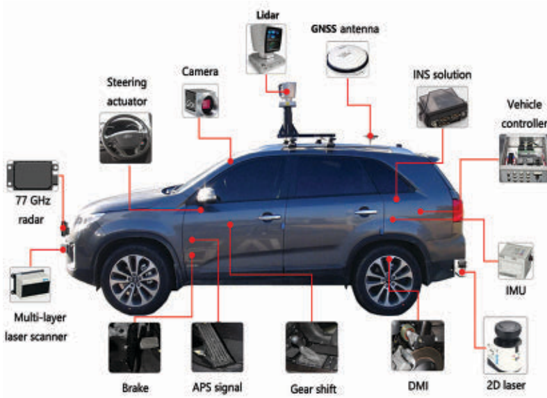
Figure 2. Sensors on a typical autonomous passenger vehicle.
