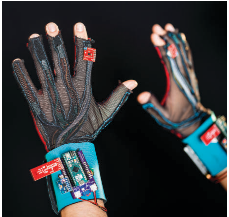
These prototype SignAloud gloves translate the gestures of American Sign Language into spoken English.
