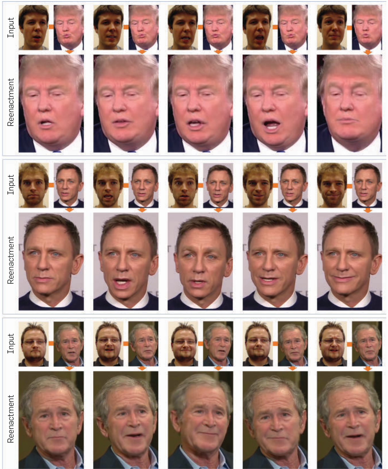
Figure 5. Results of our reenactment system. Corresponding run times are listed in Table 1. The length of the source and resulting output sequences is 965, 1436, and 1791 frames, respectively; the length of the input target sequences is 431, 286, and 392 frames, respectively.
