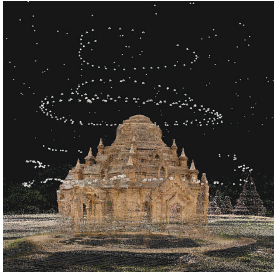
Capturing photogrammetric data for the digital reconstruction of a badly damaged temple in the ancient city of Bagan, in central Myanmar.
