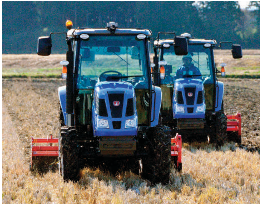
A robotic tractor (left) cultivates a field alongside a tractor operated by a human, during a demonstration in Fukushima, Japan.
