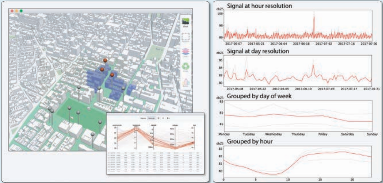
Figure 3. (left) Interactive 3D visualization of a New York neighborhood using Urbane. By selecting specific sensors (red pins) and buildings (purple) researchers can retrieve and visualize multiple data streams associated with these locations. (right) SPL data at various resolutions and time scales retrieved using the time lattice. Each sub-figure reflects different individual (gray) and aggregated (red) sensor data for the three sensor units highlighted in the left plot.
