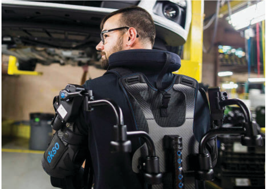
A Ford worker wearing the EksoVest, which provides lift assistance for repetitive overhead tasks.
