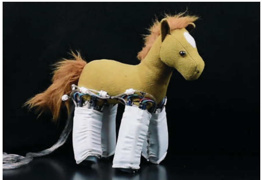
“Robotic Skins” technology developed by Rebecca Kramer-Bottiglio and colleagues at the Yale School of Engineering & Applied Science enables novel designs for robots that can move more freely.
