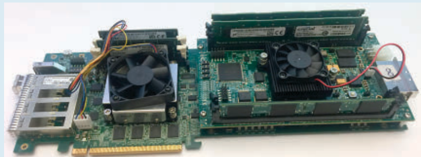
Figure 5. A prototype programmable SSD developed for research purposes.
