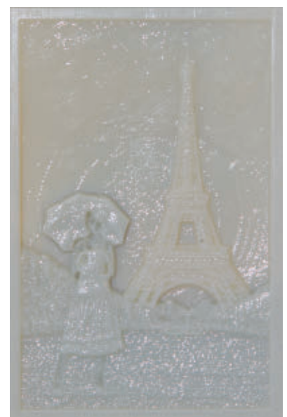
Figure 2. The front face of the postcard (left) is texture mapped using a foreground image. The back (right) displaces the surface to create a spatially varying transmission according to a combined foreground and background image. The result is a hidden background image, which only appears when backlit (center).
