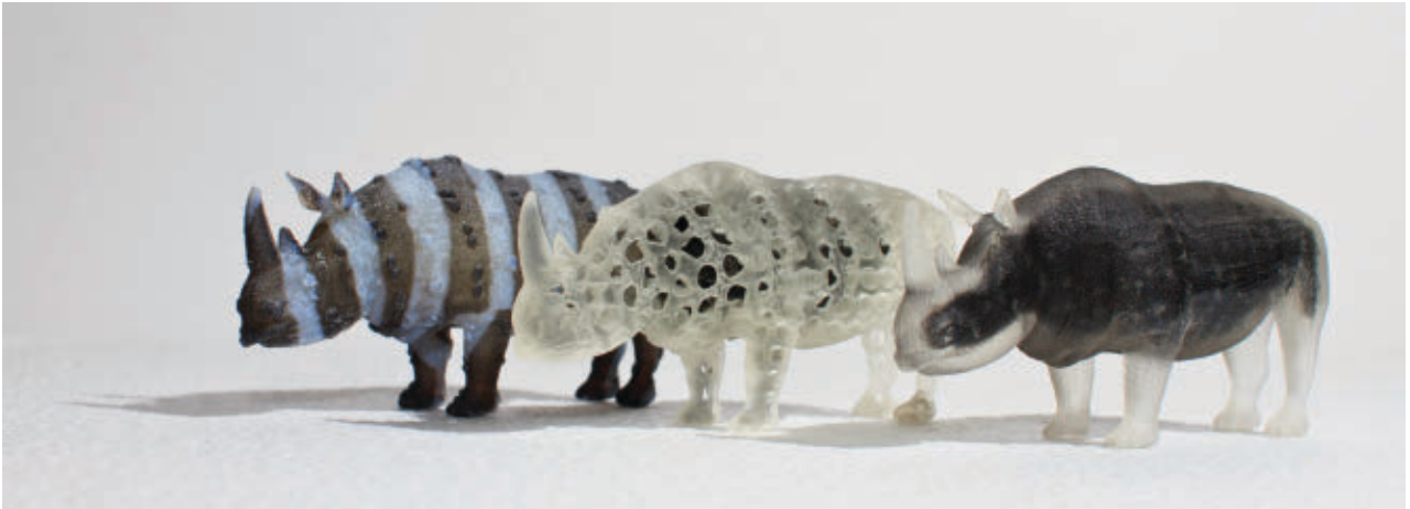
Figure 5. Three rhinos defined and printed using OpenFab. For each print, the same geometry was paired with a different fablet —a shader-like program that procedurally defines surface detail and material composition throughout the object volume. This produces three unique prints by using displacements, texture mapping, and continuous volumetric material variation as a function of distance from the surface.
