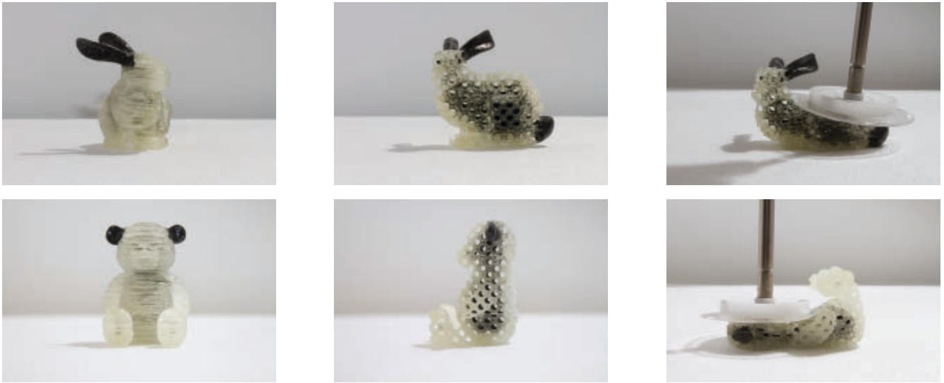
Figure 7. A procedurally defined foam material makes the bunny and bear squishy. Color and squishiness vary procedurally over the models.
