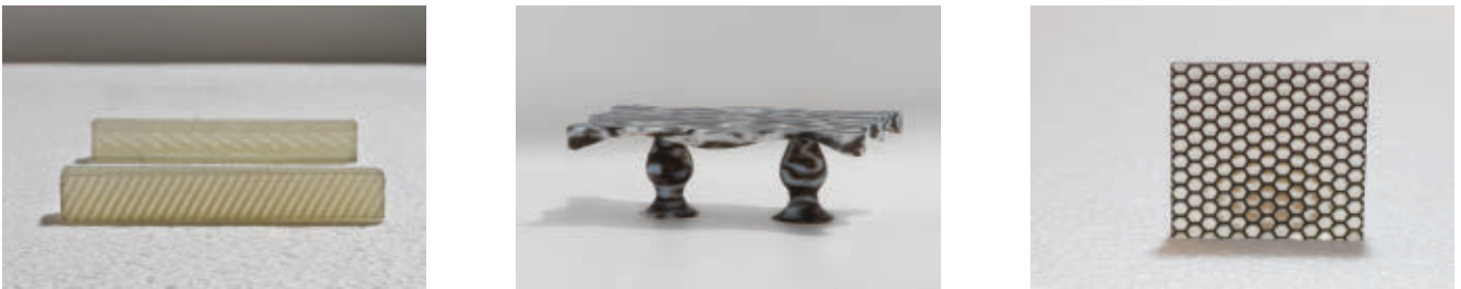
Figure 8. Left: procedurally defined materials with anisotropic mechanical properties. Center: Marble-like material generated using Perlin noise. Right: Procedurally defined and fully parameterized aspherical microlens array with baffles.
