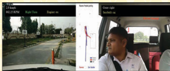
Figure 2. Tracing the trajectory during a parallel parking test (blue = forward, red = reverse) using a windshield-mounted smartphone, which analyzes outside and inside views concurrently. Source: HAMS project; http://bit.ly/2ZseQXC .
