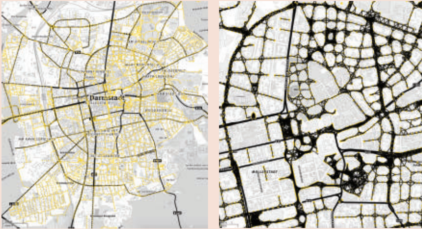
Figure 3. Geographic density of public street lamps in urban areas (left) and resulting wireless mesh networks ( d = 50\text{m} ) of interconnected inner-city street lamps (right), presented by the example of Darmstadt (Germany).
