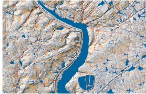
Figure 1. A terrain-flood query over a region of Philadelphia, PA, USA. The areas marked in blue are flooded, with regions that water flows over marked in orange.
