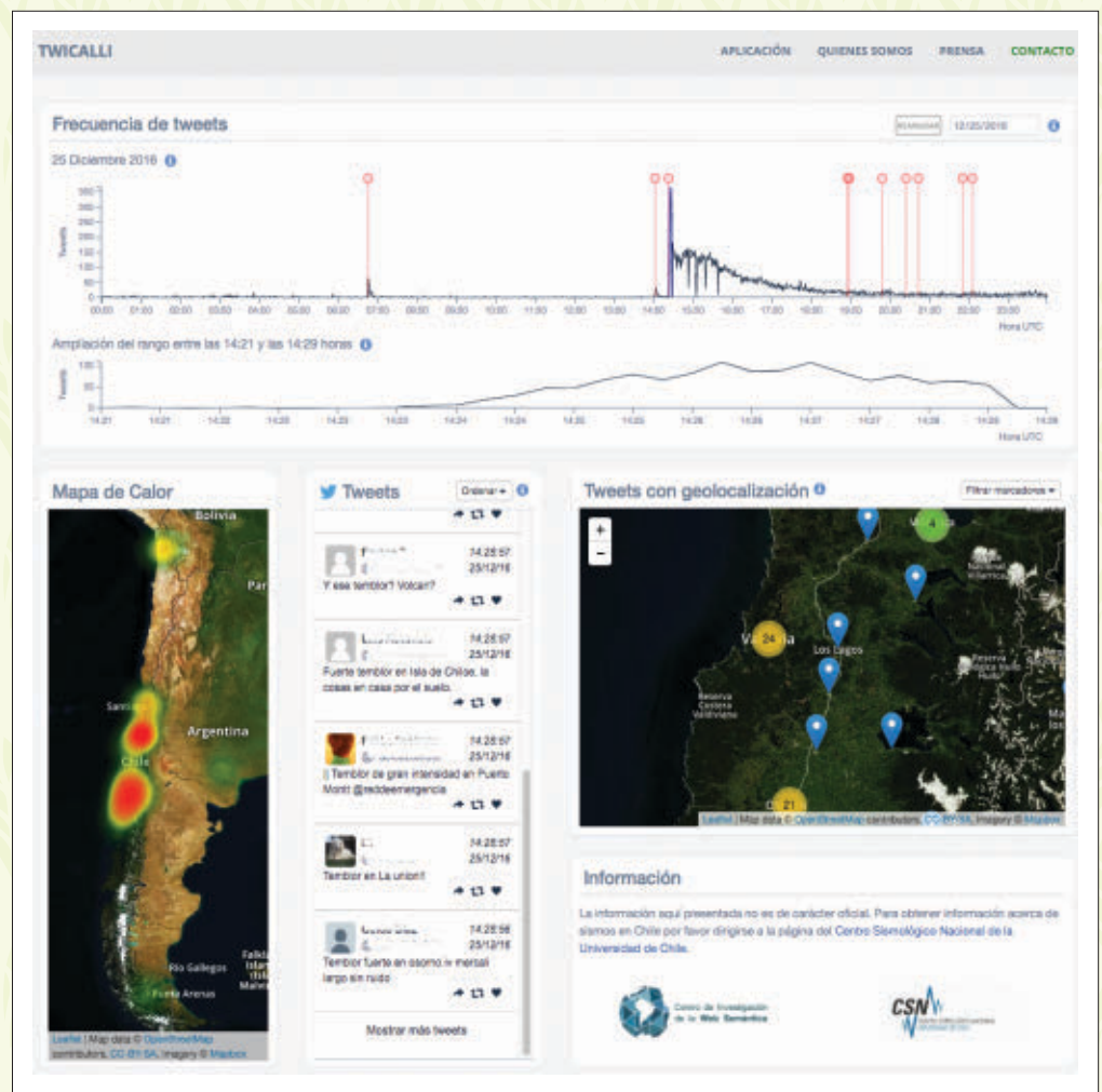
Figure 1. Twicalli interface showing a large earthquake in Chile on December 25, 2016 and its aftershocks. (Top right) Shows the frequency of earthquake-related messages per minute. (Left) Shows a heat map of geographical message density distribution. (Bottom center) Displays user messages. (Bottom right) Shows fine-grained geographical message navigation. Image courtesy of Jazmine Maldonado.
