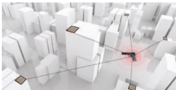
Figure 15. Outdoor SATURN patches can sense and communicate gunshot sounds to indoor transceivers for real-time triangulation.
