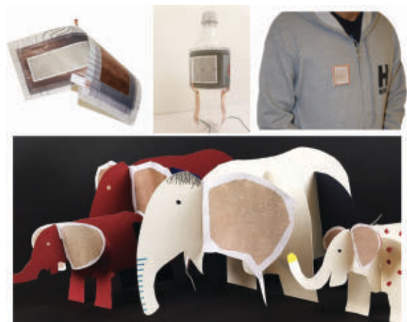
Figure 12. SATURN is flexible and can be made in different shapes and sizes, allowing instrumentation of everyday objects such as a soda bottle, shirt, and paper crafts.
