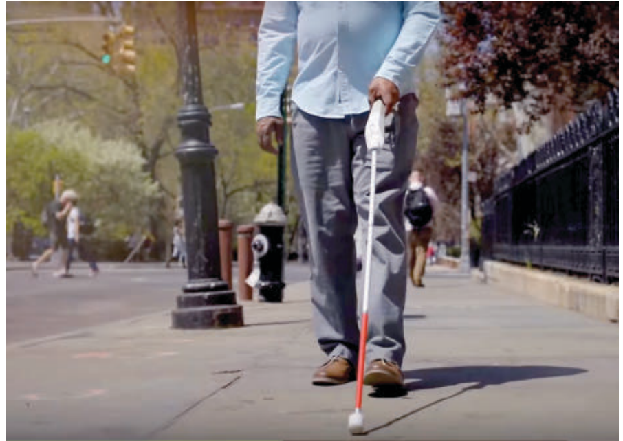
The WeWALK Smart Cane detects objects in the vicinity and provides audible alerts to prevent collisions.
