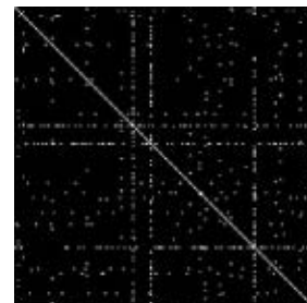
Figure 4. The nonzero elements in AA^T for the example of Figure 3.
