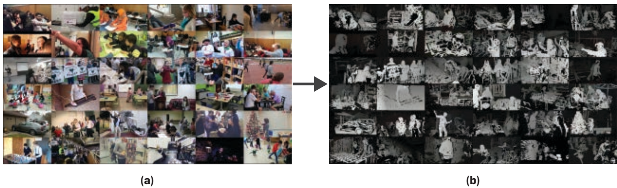
Figure 8. Our model takes as input an RGB frame, a human segmentation mask, masked depth computed from motion parallax (via optical flow and SfM pose), and an associated confidence map. We ask the network to use these inputs to predict depths that match the ground-truth MVS depth.
