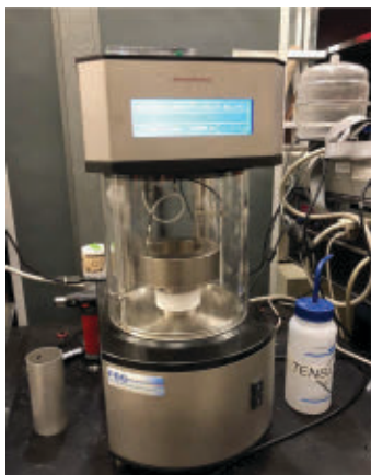
Figure 7. Digital tensiometer with a resolution of 0.1 mN/m for measuring ground truth of surface tension (Model: Dataphysics DCAT 11 9 ).
