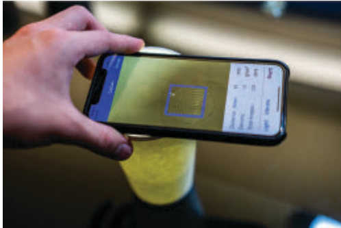
Figure 1. CapCam setup: the phone is placed on a paper cup. Capillary waves are generated by the vibro-motor inside the smartphone. Then with the flashlight, the camera of the phone can capture a bright-and-dark pattern, from which we can calculate the surface tension of the liquid.
