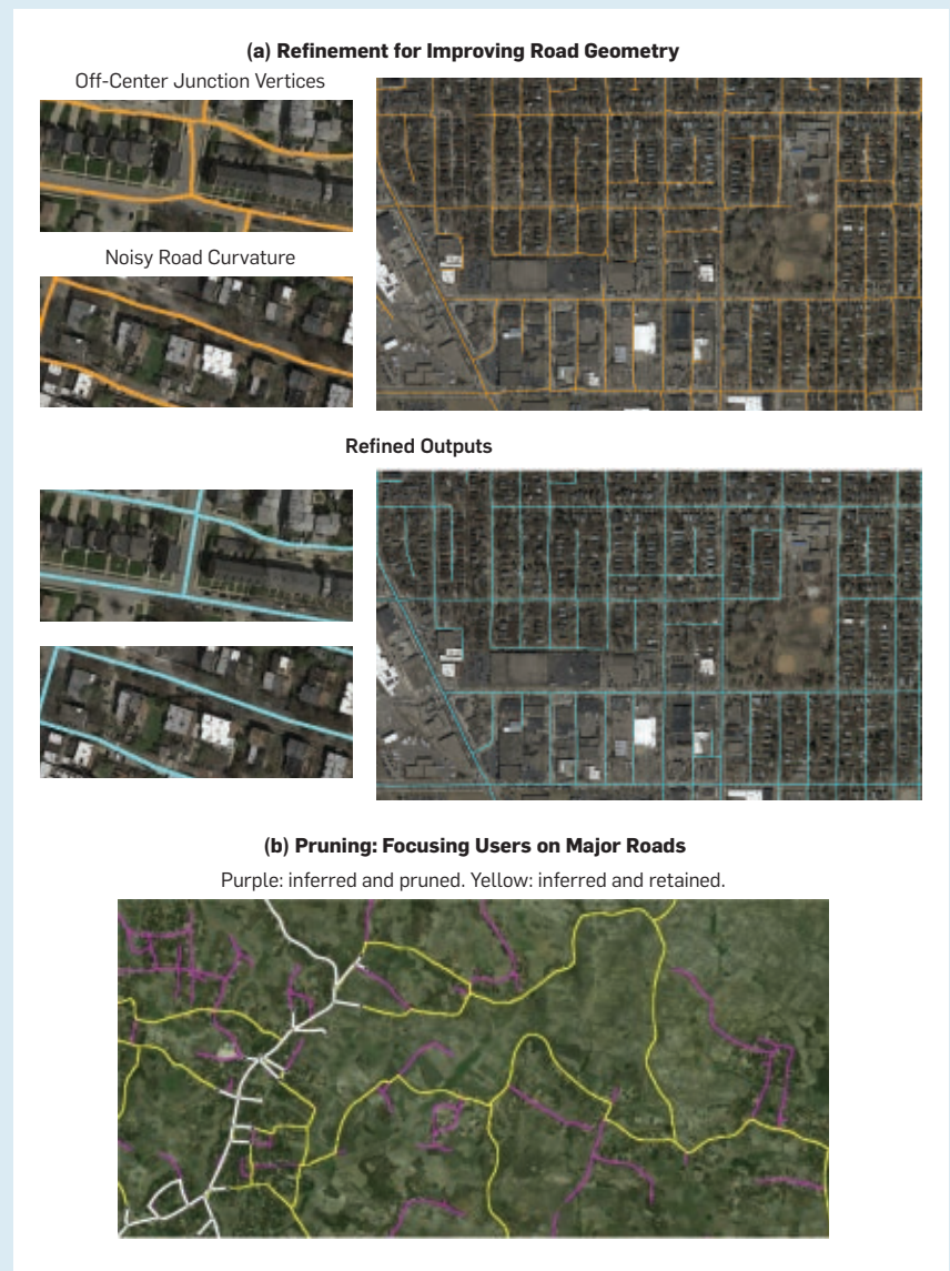
Figure 5. (a) Road networks before refinement, in orange, contain geometric abnormalities. The refined road networks, shown in blue, clean up these noisy features. (b) Our human-in-the-loop map-editing system employs a pruning algorithm to eliminate residential and service roads and focus the user on adding major roads to the map. Pruned roads are shown in purple and the remaining roads in yellow.
