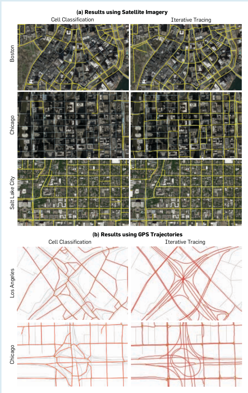
Figure 3. Qualitative results comparing iterative tracing to prior cell classification approaches shows (a) road networks inferred from satellite imagery, and (b) road networks inferred from GPS trajectories. We show inferred roads in the foreground and OpenStreetMap data in the background.
