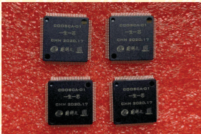
The 64-bit NutShell RISC-V processor designed by students from the University of the Chinese Academy of Sciences.
